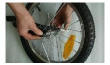
Step 3: Connect loading frame(1) and the fork with wheel by connect nut(10) as per below images:
