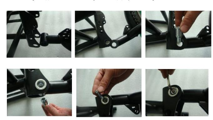
Step 4: Install the damper(6) on the loading frame(1) as per below images:
